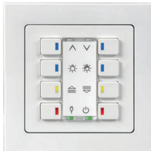
The Piazza series are simple and timeless in design and suitable for mounting in standard installation boxes. They are available as variants with 2, 4, 6 and 8 keys, with status LED for each key (RGB version) or without. The scope of functions covers all the standard functions required, such as switching, dimming, value setting, incremental value setting, shutter, scene control, setpoint shift, operating mode setting, presence, fan control, individual keys (on, off, toggle).
