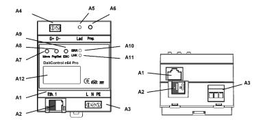
A1: RJ-45 plug for Ethernet connection
