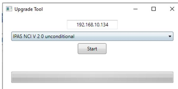
To start the upgrade, enter the IP address of the device that you would like to upgrade. Double-click on the displayed IP address (here 192.168.10.134) to open the entry field.
