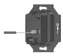
To dismount a connected plug, please press down the lever on the locking catch.
