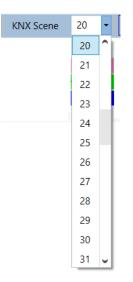
In the example above, the selected DALI scene can be invoked object value 19 (KNX scene 20), respectively programmed by value 147. Please note that the assignment hast o be unique. If different DALI scenes are assigned to the same KNX scene only the first DALI scene is activated / programmed.
