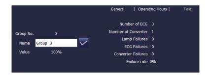
In addition to the number of devices and converters and the individual error types, the total error rate within a group is shown. Please remember that the rate is calculated as a percentage of the total number of ECGs and converters in the group. Use the Name field to enter a user-friendly name for the group. The maximum number of characters is 10. Press the  $\sqrt{-button}$  to confirm your entry. The name is now saved on the gateway and loaded into the ETS during the next synchronisation.
