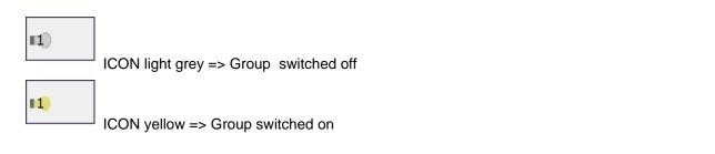
If you switch a group or ECG via the website, its status is automatically updated and displayed on the site. However, if the switch command was initiated externally via a KNX telegram, the status is not automatically updated. To display the correct status, press the refresh button or re-load the web page.
