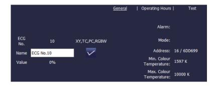
On the General page the first line shows the ECG number as well as the possible sub-types for DT-8 devices. For all other ECG device types (DT-0..DT-7) the entry remains empty.
