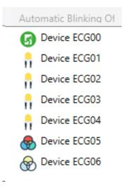
To identify the devices, switch the corresponding lamp on and off. If you select an ECG and press the right mouse button, a context menu appears from which you can select the required function.
