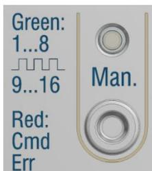
The manual mode ends automatically 60 seconds after the last time the button has been activated.
