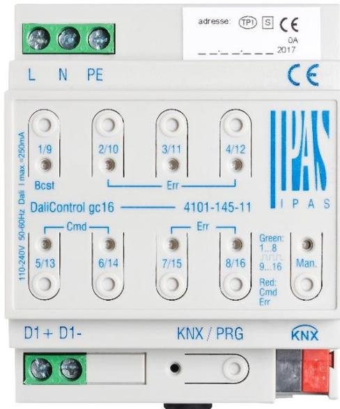
The buttons and LEDs are accessible without having to remove the cover. During KNX bus operation and in the absence of any errors, all 9 LEDs are switched off. If the gateway detects an error (e.g. a faulty lamp or KNX failure), only the LED on the Man. button lights up in red and flashes quickly. During programming (e.g. during installation) all LEDs light up in red and flash slowly.
