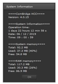
The menu item **System Info** provides the user with information about currently available memory space, the software version and the length of time the device has been running since the last start-up.
