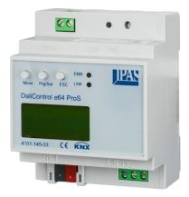
The device transforms switching and dimming commands from the connected KNX system into corresponding DALI telegrams, or status and event information from the DALI bus into KNX telegrams.
