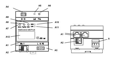
A1: 2x RJ-45 plug for Ethernet connection integrated Switch
