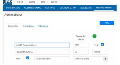
Configuration of the MQTT connection in the web interface
