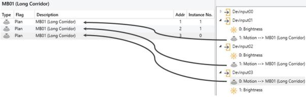
A virtual push button in the DCA can also be parameterised with up to 4 physical instances:
